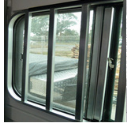
Horse float security window steel bars
